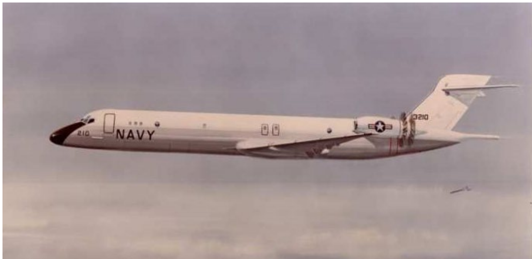
This artist's conception of the "Advanced USN Patrol Aircraft" shows an aircraft similar to the DC-9 airliner with unducted fan engines.
