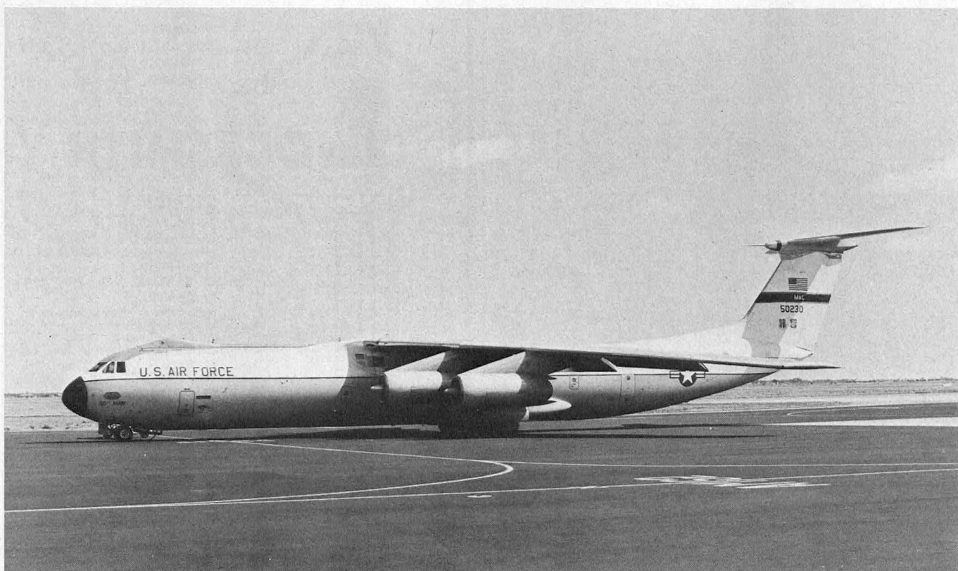
• The above photograph shows the C-141B on its recent visit to Edinburgh. The "stretched" fuselage and the inflight refuelling equipment above the cockpit can be clearly seen.
