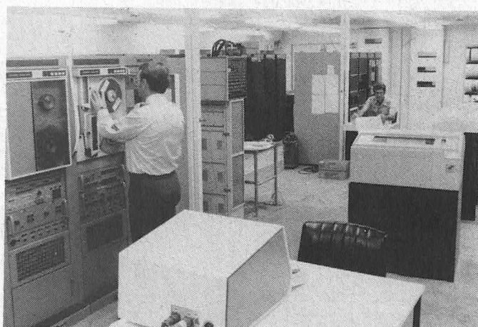
View of the CMI Computer room, where P3C programs are compiled and mission tapes loaded for replay and analysis.
