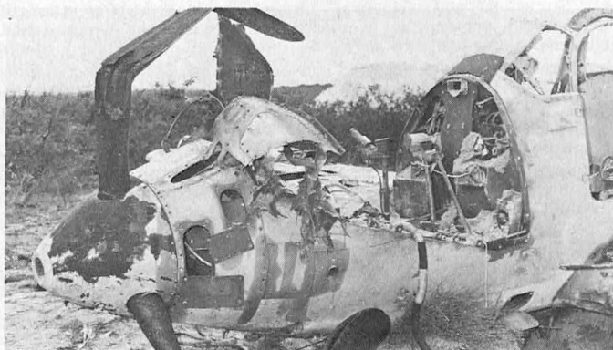
• Damage caused to the nose section of Lt. Harvey's aircraft by charges detonated to clear the corroded and highly dangerous ammunition that could not be removed by the demolition team.
